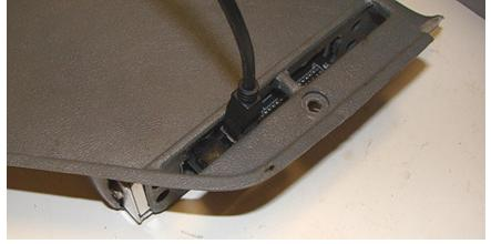
9) Reinstall ECU in kick panel, you should be able to plug in the USB cable through the vent slot.
