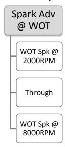
On the Spark Advance Page is where you set the WOT timing. This function is only operational with the Extreme G chip. All other chips do not use this feature. These will be set to the lowest timing by default, which is 15 degrees.
