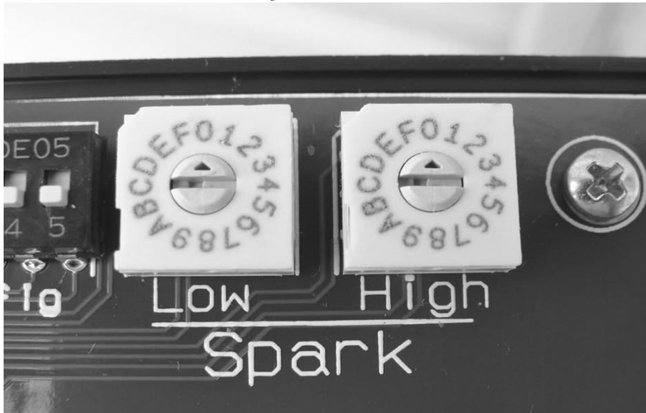
Be careful with these settings! Make sure you are monitoring for knock. These settings add or subtract from you chip's base timing if you have a compatible chip. "Low" is 0psi boost and lower, "High" is 10psi boost and higher (full throttle).
